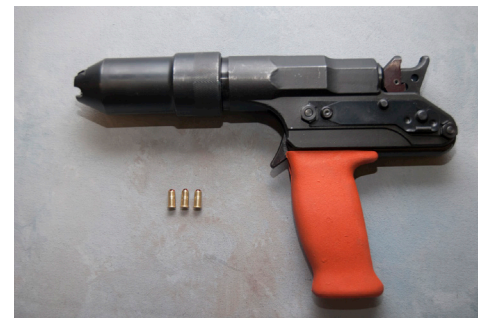
Penetrating captive bolt and charges
